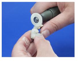
For this type of application we can also recommend using our special Buffing Wheel for prepolishing, a Buffing Wheel or a Lathe Brush with cotton cloth together with wet pumice.
